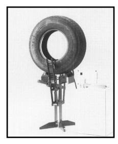
Place tire on inspection unit. Spreading the beads.
