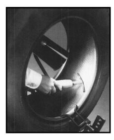
T-probe follows inner circumference of the tire; touching the surface of the innerliner.
